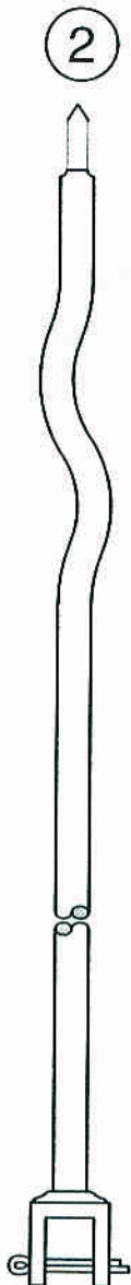
STAINLESS STEEL ROD WITH WELDED STAINLESS STEEL CLEVIS AND COTTER PIN KINKED
